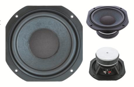
The BM220.1 features a symmetrical field magnet, dual rear suspensions and an extended voice coil for exceptional bass performance at high power levels. It is suitable for use singly or in multiples in compact high power systems where space is at a premium. Operation in a 5 litre sealed box offers an exceptional combination of bass punch, sound level and reliability.
