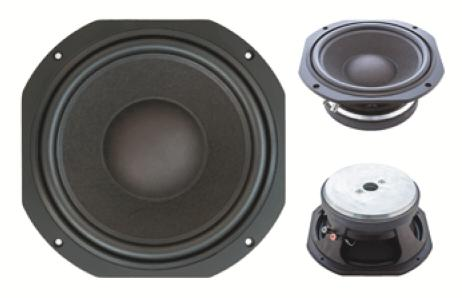
The B2500.1 uses a massive magnet with symmetrical magnetic field and extended pole for maximum linearity. Matched dual rear suspensions maintain stability at high power levels. The cone is exceptionally rigid ensuring true piston integrity. The B2500.1 is the ultimate 250 mm high power studio bass driver. This unit is intended for state of the art studio systems where dynamic range and analytical clarity are essential.
